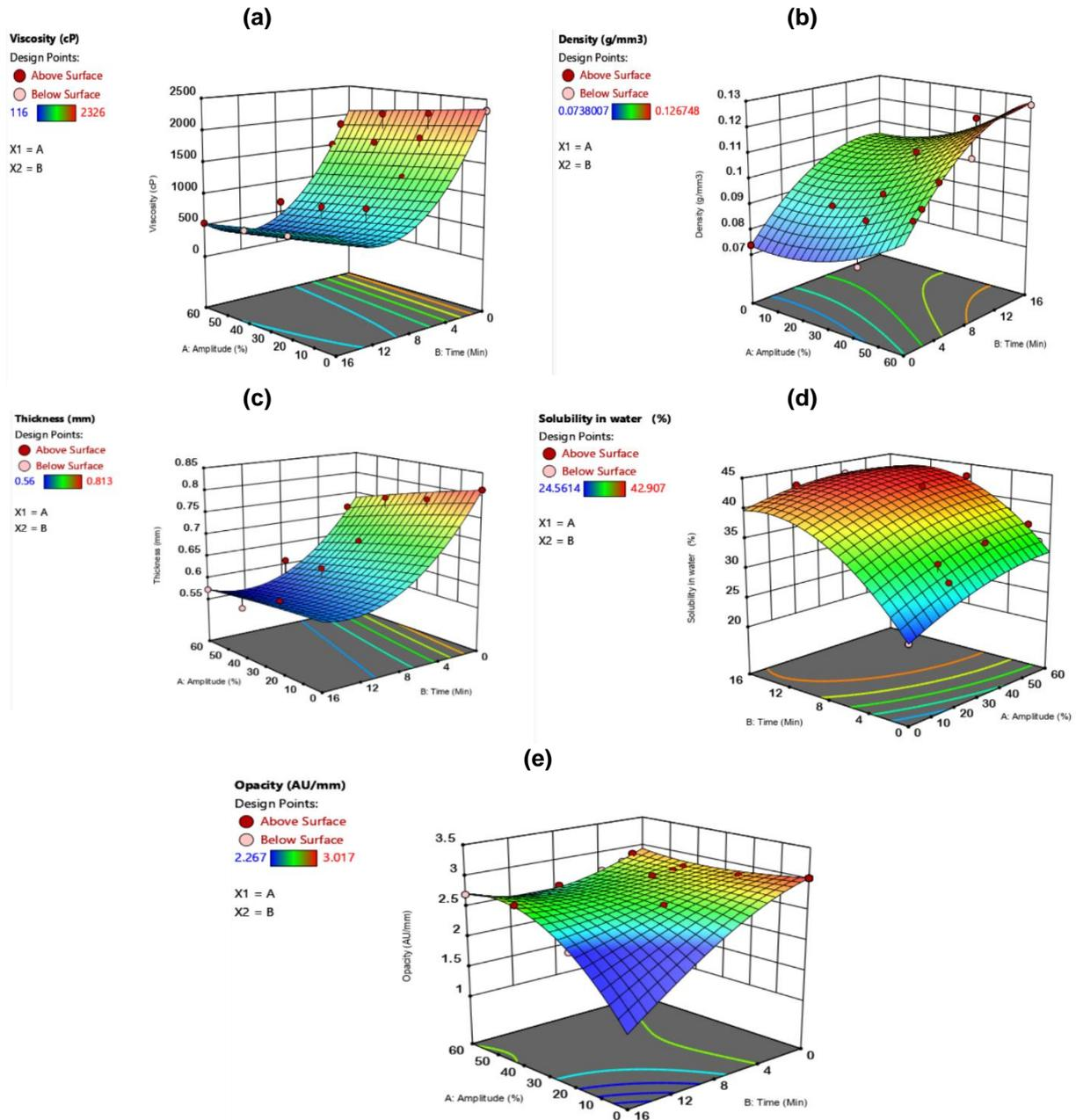
**Fig. 4. Response surface plots showing the impact of variables on: a) Viscosity of casting solution, b) Density, c) Thickness, d) Solubility in water and e) Opacity of Composite biodegradable cup**
