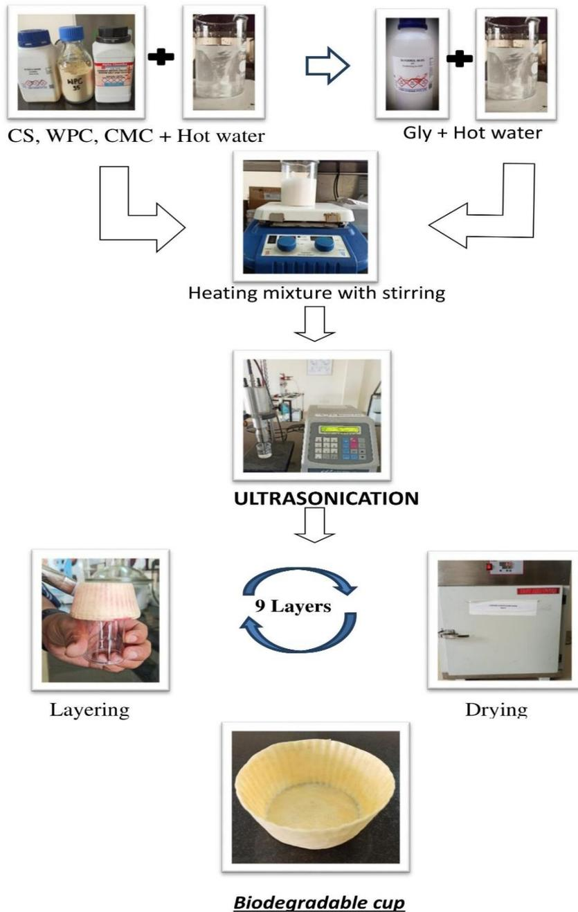
**Fig. 1. Visual representation of method for development of biodegradable cup**
