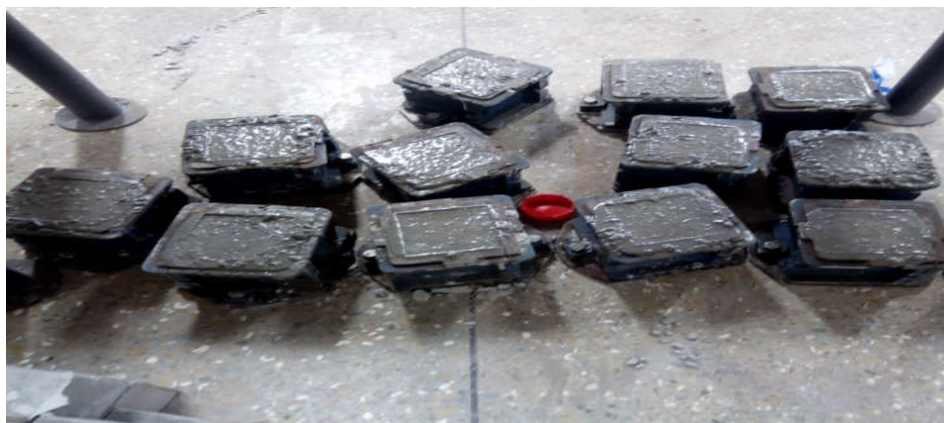
Fig. 1. Concrete cubes in a mould
